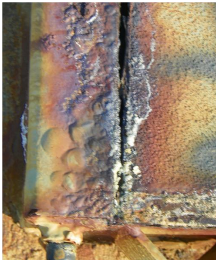
Photos above and at the right are close-ups of corrosion on the two-year-old utility vault doors in Van Buskirk Park.
